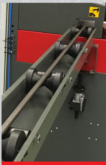
Roller conveyer for 3 or 6 metres
